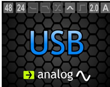
The default home screen view consists of three components. The currently active input is displayed at the center.
