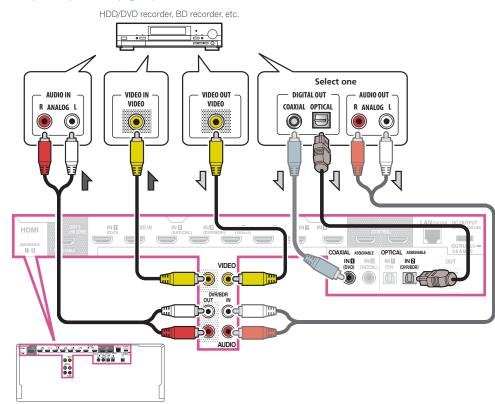
In order to record, you must connect the analog audio cables (the digital connection is for playback only) (page 78).
