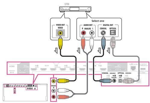
If your set-top box is equipped with an HDMI output terminal, we recommend connecting it to the receiver's HDMI SAT/CBL IN terminal. When doing so, also connect the receiver and TV by HDMI (see <u>Connecting using HDMI</u> on <u>page 29</u>).
