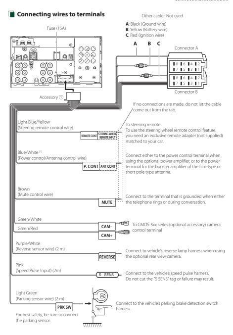
[1] [2]: Blue/White wire is provided two wires, [1] and [2]. Blue/White wire total output ([1] + [2]): 12 V == 350 mA
