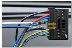
12. Insert the terminals of the cables from the supplied T-Harness into the connector from the instrument cluster.
