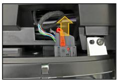
5. Remove the connector from the instrument panel.
