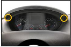
1. Remove the two screws of the instrument panel cover.
