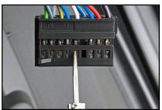
9. Release the terminals of the CAN cables with the suggested release tool.
