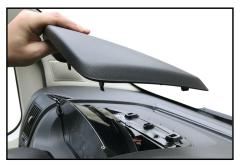
3. Now remove the cover completely from the instrument cluster.
