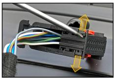
6. Release the locking clips of the connector housing.
