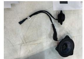
**5** Secure all Alpine speakers to the dash by Re-installing all remaining factory T20 Torx. After speakers are mounted Install the dashboard speaker cover panel by applying uniform pressure to engage the factory clips.
