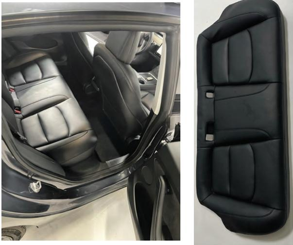
**2** Locate the low voltage 12V battery posts in the rear seat passenger compartment (Under the seat) Use a socket to remove the battery post hardware nuts
