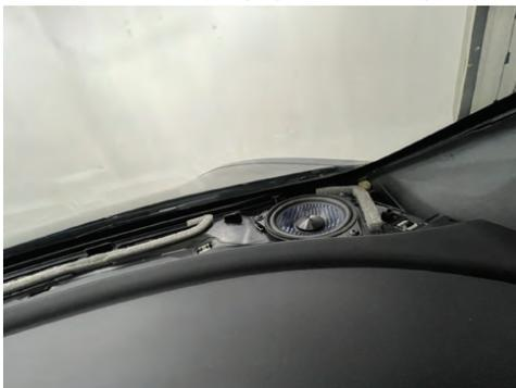
**6** Re-install dash side cover "A" followed by pillar cover "B" at both sides of vehicle.
