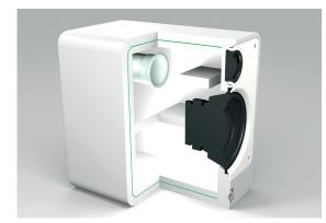
The 'cabinet within a cabinet' Gelcore™ construction dramatically reduces resonances and colouration.
