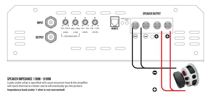
We recommend using minumum 8 Ga speaker cables to acquire the intended performance & efficiency. Run the speaker cables from your speakers to the amplifier's mounting location.
