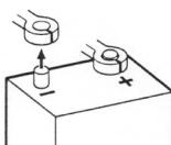
**Warning:** Never touch or route cables near high-voltage (orange) harnesses. Do not open or modify any airbag/SRS connectors. Place the disconnected terminal in a secure and isolated location away from any possible connection belonging to the battery/power source system.
