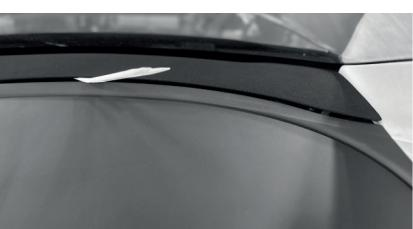
To remove the speaker cover panel, all clips need to be released. Pull upwards to detach and expose the midrange speakers.
