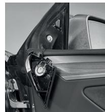
The OEM tweeter is snapped into a holder in the tweeter cover panel. Use the pry tool or small flat head screwdriver to remove it.
