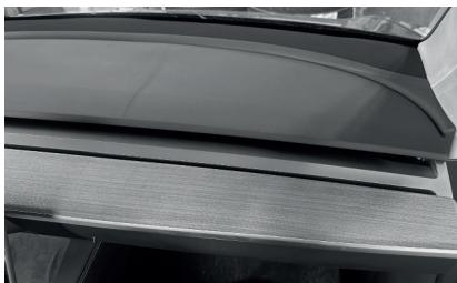
To remove the speaker cover panel start by removing the A-pillar covers on both left and right sides. Use the included pry tool. The weather gasket can be moved back for easier access.
