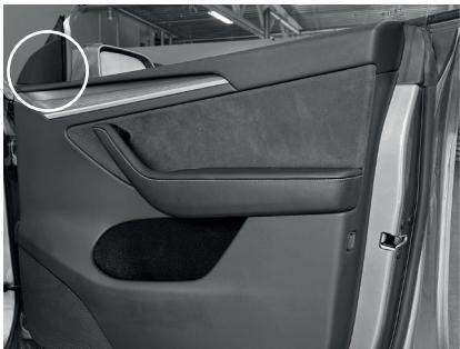
Start by removing the tweeter covers. Use the pry tool and be careful. The clips can be hard to remove. Take it easy and use minimal force.
