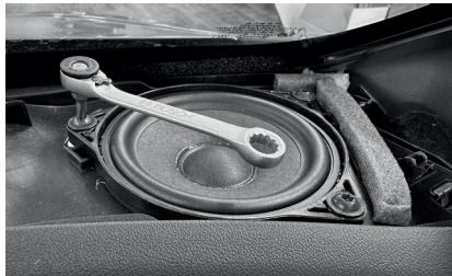
Unscrew them and store the screws in a safe place, for later use when reinstalling the door panel.
