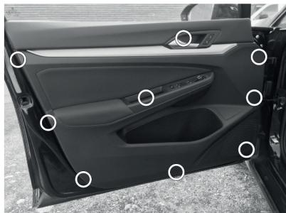
Typically the clips/screws are located around the perimeter of the door panel; however this varies depending on the vehicle. Sometimes they are hidden under a plastic cover or behind another panel which can be removed using the included pry tool.
