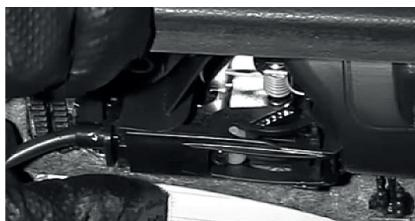
There are often several electrical and mechanical connectors installed in the door panel. Disconnect any connections and remove the door panel.
