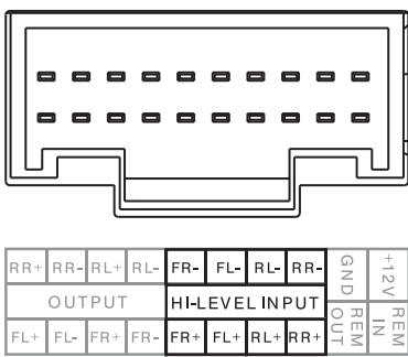
The high-level input connector wires follow the standard DIN-color coding. However, the car's wiring loom may use different color codes. When using high-level inputs, the amplifier's turn-on signal is derived from the high-level input itself, eliminating the need for a separate remote wire.
