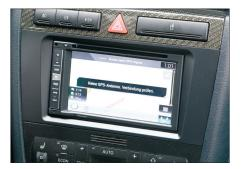
8. Place facia plate on dash board to finish installation
