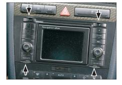
Insert radio release keys made for cars with horizontal release slots - e.g. ACV part-no 181320-02\*
