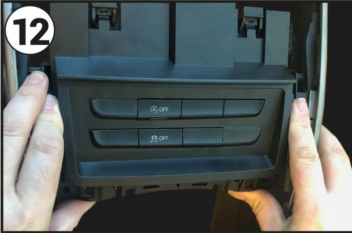
With the new Button Relocation Panel fully assembled, install it into the opening where the ashtray originally sat. Before fully placing, make sure to re-connect both MMI button connectors.
