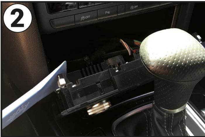
**2** Using the Bojo tool again, pry away and unclip the bottom HVAC panel. Once loose, disconnect the panel connectors and place to one side.
