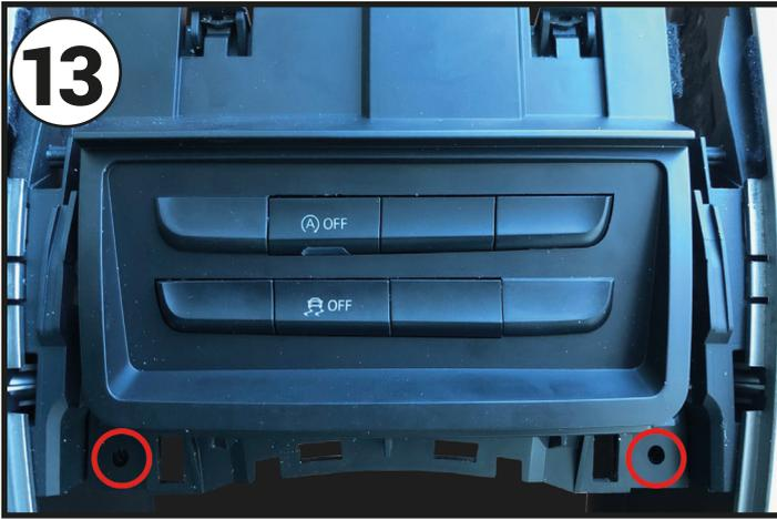
Once the Button Relocation Panel is seated properly, screw the panel down into place using the OEM screws.
