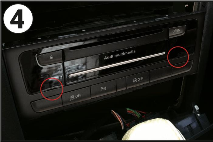
Using a pair of radio release keys (e.g. **CT22AU01**) remove the head unit. When free, disconnect all the wiring.
