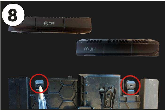
Take the OEM head unit in hand and gently remove the buttons by means of releasing the surrounding plastic.
