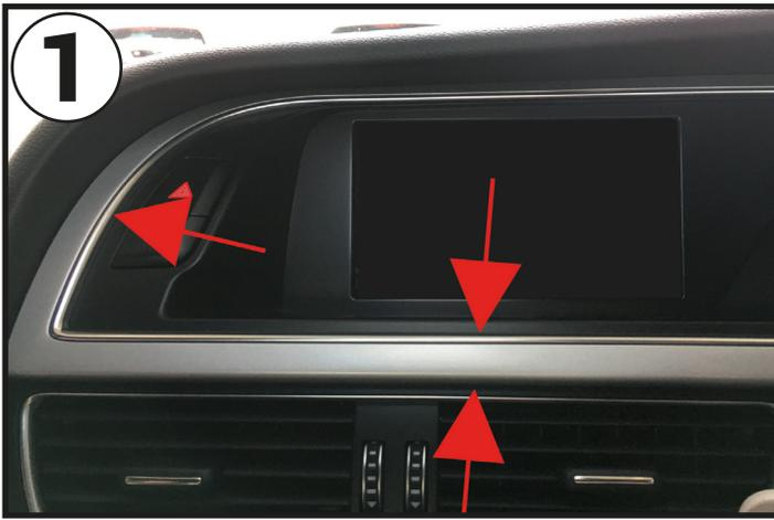
**1** Begin by using a Bojo tool (or similar variant) to pry away and unclip the trim that surrounds the top screen. Once loose, disconnect the hazard switch connector and place to one side.
