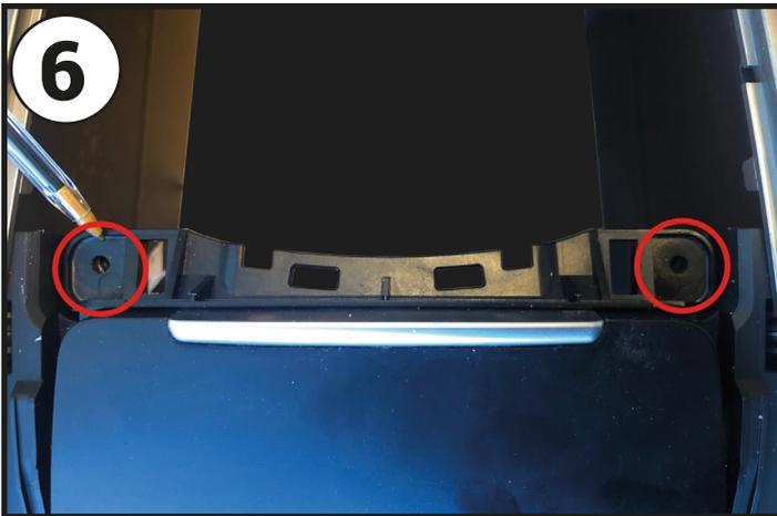
Remove 2x 8mm screws located toward the bottom of the ashtray panel (*see image reference*). When free, carefully lift and pull the ashtray pocket up out of the dashboard.
