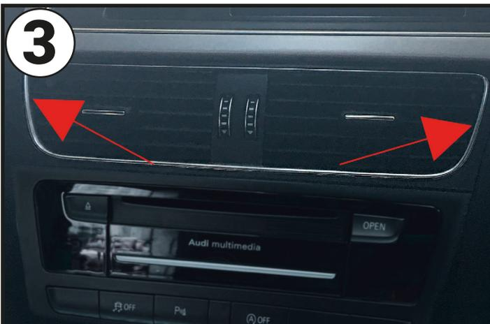
**3** Using a pick tool, insert it in between the fan blades and release the spring clips. Once free, remove and place into storage.
