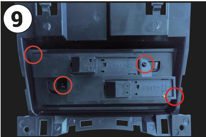
Install the OEM head unit buttons into the new Button Relocation Bracket. Further proceed to install this button and bracket combination into the back of the new Button Relocation Panel (see *image reference*).
