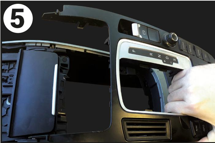
Pull the gear stick cover up and then firmly pull on the centre gear panel. Disconnect both wires and put to one side.
