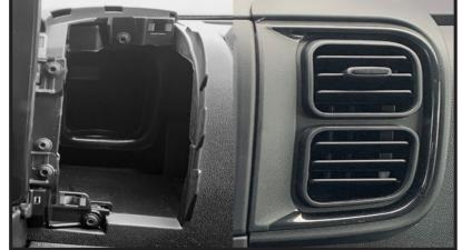
With the air vents removed, you will then 3. need to undo the 4x screws that surround the main fascia. Once undone, simply pull the fascia away from the dashboard.
