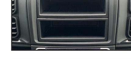
Use the panel removal tool to unclip the 2. entirety of the side air vents. Once free, simply pull them out of the dashboard and set them to one side.
