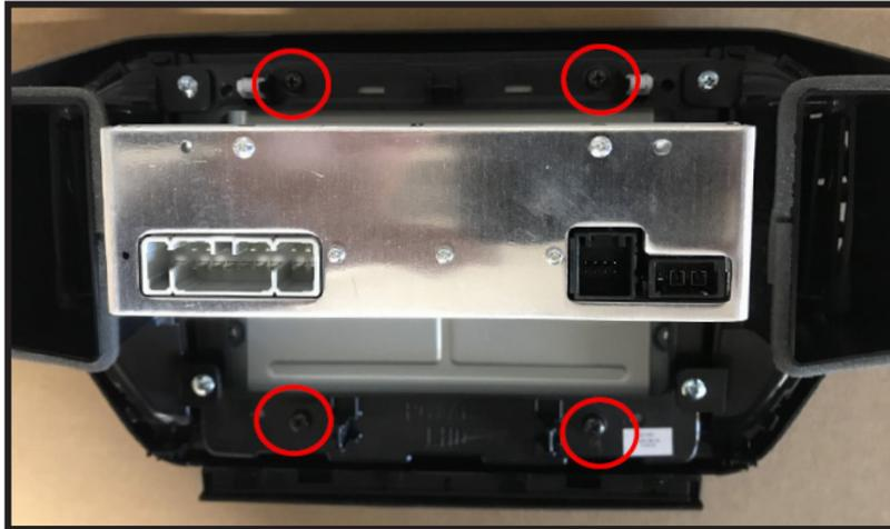
Undo all four screws located on the rear of the main fascia panel. These screws will disengage the air vents and trim from the main single DIN unit/touch screen.
