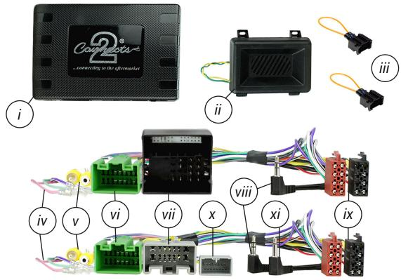
i. Interface Box ii. Speaker Module iii. MOST Loops (x2) iv. Flying Wires
