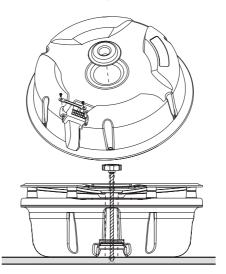
**3.** After the connection, place in the spare wheel active subwoofer to the spare loction, make sure to press down the subwoofer firmly.
