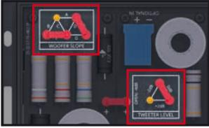
The crossover allows to optimize the level of the connected tweeter as well as the adjustment of the lowpass filter slope to the connected COMPOSE midrange, midbass or woofer internally by repositioning level jumpers. Therefore open the crossover housing, pull the appropriate jumper straight upwards and reinsert it to the desired position.
