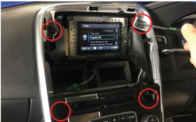
With the trim panel and the CD slot panel removed, proceed to undo the 4x Torx screws highlighted. Once undo, pull the whole panel forward and disconnect all of the wiring.
