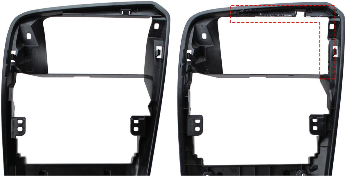
The highlighted section of dashboard frame will need to be cut in order to allow for a new double DIN unit to sit in place correctly.
